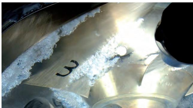
IEC60193 Cavitation Test at EPFL: Reduced Scale Physical Model of a 120 MW Kaplan turbine
