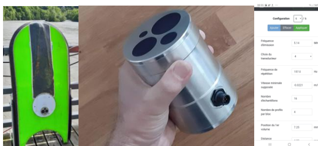
Figure 1 : From left to right: the UB-SediFlow on a floating board, the acoustic module and the user interface
